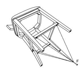
STEP 6 Place stool upright on a Level floor and press firmly down to even out of the legs, Once legs are Level use a ALLEN WRENCH to tighten all Bolts ( C , D )
