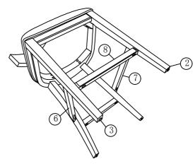
NOTE: Leave BOLTS loose by 1/4 turn when | NOTE: Do not add WOOD SCREWS (F) until STEP 5.
